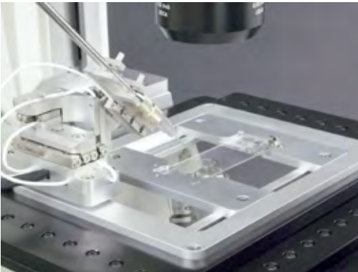
A four axis micromanipulator allows positioning of tools with nanometer precision in front of the objective lens.
