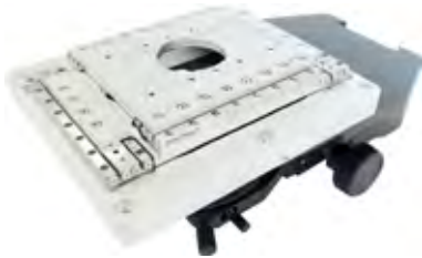
The SOM-MS-CST-SLC-1780 stage was designed to fit in all Olympus® BX series microscopes.
