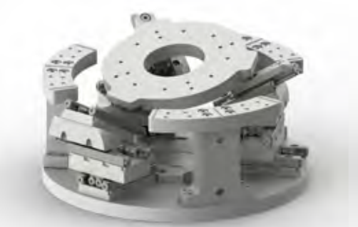
SMARPOD 110.45 in a deflected pose.
