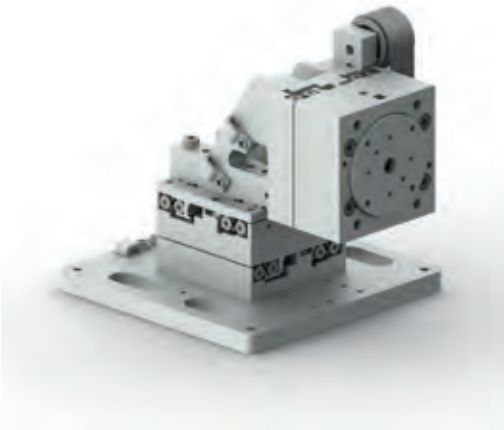
XYZR-XYZ SLS32:32 Z SRP32:11: A 4D positioning system consisting of three SLS-3232 linear stages and one SR-3211 rotation stage
