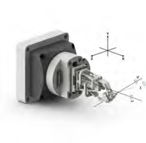
The six degrees of freedom of the SMARGON positioning system.
