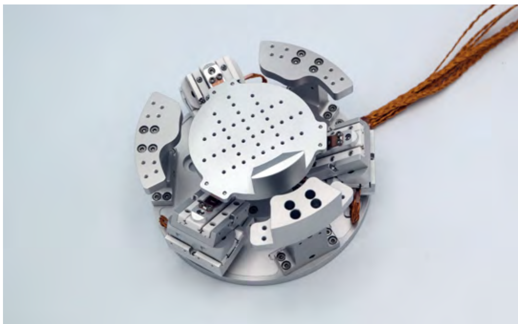
A modified SMARPOD 110.45 in a non-magnetic version for use in ultra-high vacuum environments.
